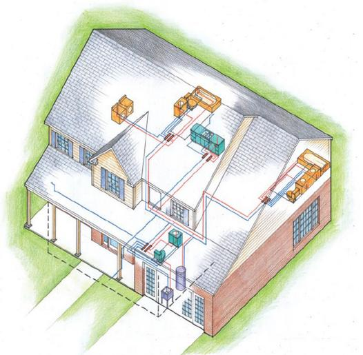
PEX plumbing systems can be installed as Trunk & Branch, Home-run, or Zoned using remote manifolds as shown in this illustration.
